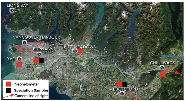
**The Lower Fraser Valley visual air quality monitoring network.** Arrows reflect the "line of sight" (or the direction toward which the camera is facing) for each camera featured on clearairbc.ca. For example, the Abbotsford camera takes photos of Mount Baker to the southeast.
